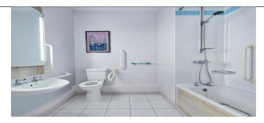
The clear door opening width of the bathroom door is 36" (91cm). The height of the WC from floor to seat is 19" (48cm) and the transfer side when looking at the WC is to the left. The height of the washbasin 29" (73cm) and there is clear space under the basin.
